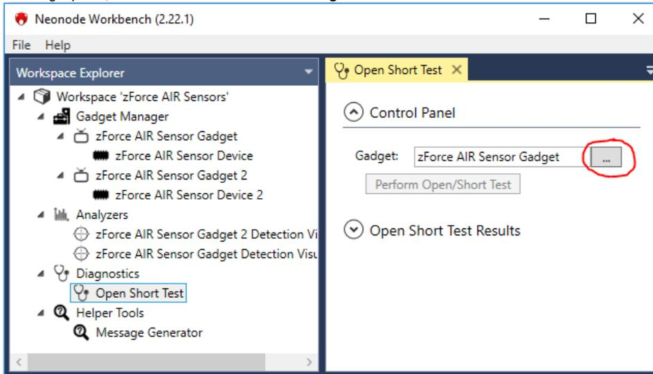
3. Click the button to perform an open short test on all photo diodes and laser diodes.
